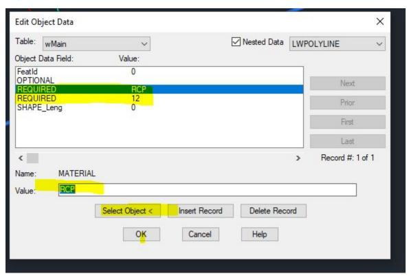
These can be done individually or if multiple objects have the same values, they can all be applied at once. Table 1-1 shows the list of water line & storm pipe materials required by the City. Continue this procedure until all layers have been populated with the attribute data. Optionally the data can be populated thru the properties dialog box.
