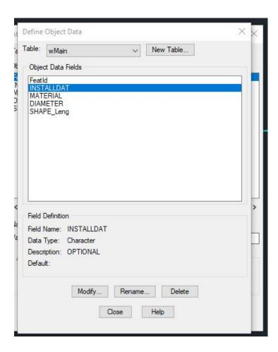
After attaching the table to the objects, the command ADEEDITDATA (ribbon: Tools – MapEdit) is used to attach the data.
