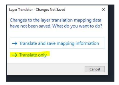
The layers in the drawing have now been renamed to the required layers. Save your drawing. Open the template file (.dwt). Insert the saved drawing file, Insert tab or type Insert on command line, then save the .dwt as a .dwg file. Do not save the template file. This will insert the object data templates into the submittal drawing and preserve the template file for future use.
