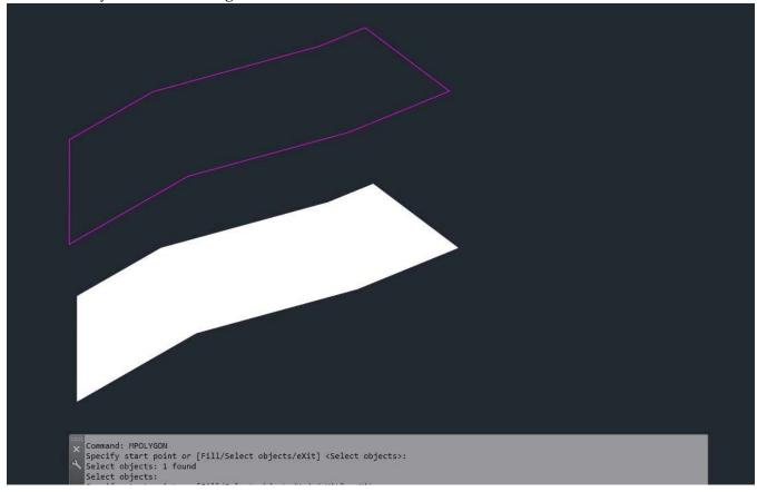
When all data has been attached to objects and mpolygons created, shapefiles can now be created. Each layer must be individually exported; thus, layer isolation will again be used. MAPEXPORT (ribbon: Output – Map Data Transfer – DWG to SDF; change output from .sdf to .shp).
