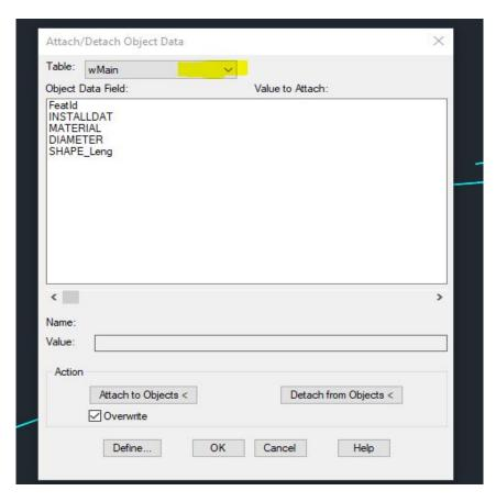
Select "Attach to Objects", then select all the mains. The command line will show the number of objects the data table attached. Notice the data field list, select a field, the Description will indicate if the attribute data is required or optional.
