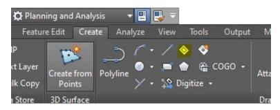
Select the closed polyline, a filled solid will be created. If not solid, then ensure the polyline is closed and try the command again.
