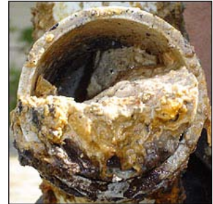
FOG build-up in a sewer pipe
