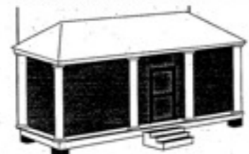
If a porch is enclosed, the architectural elements should not be covered and the material used should be transparent.
